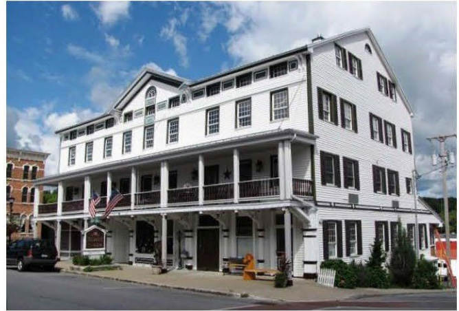
A shopfront building with pedestrian protection from sun and rain provided by a projecting second floor balcony.
