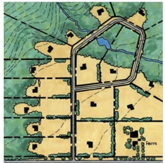
Yield Plan - Identifies the number of dwelling units that would be permitted in a conventional subdivision
